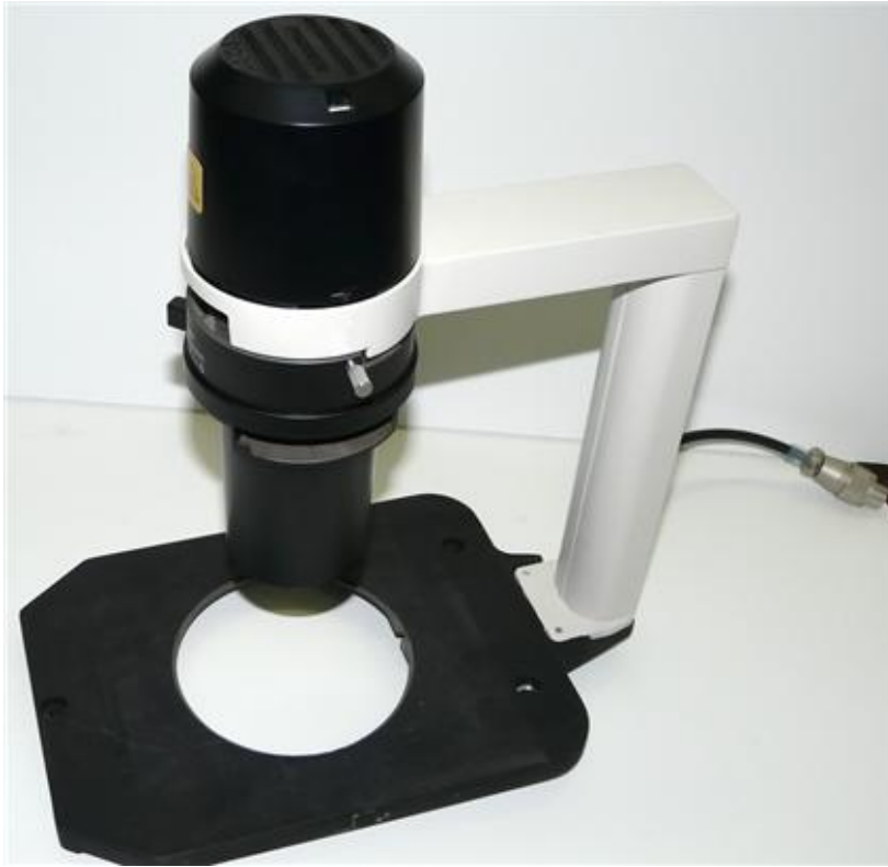
(1) Remove the lamp assembly and stage from the microscope (three screws hold it in place).
