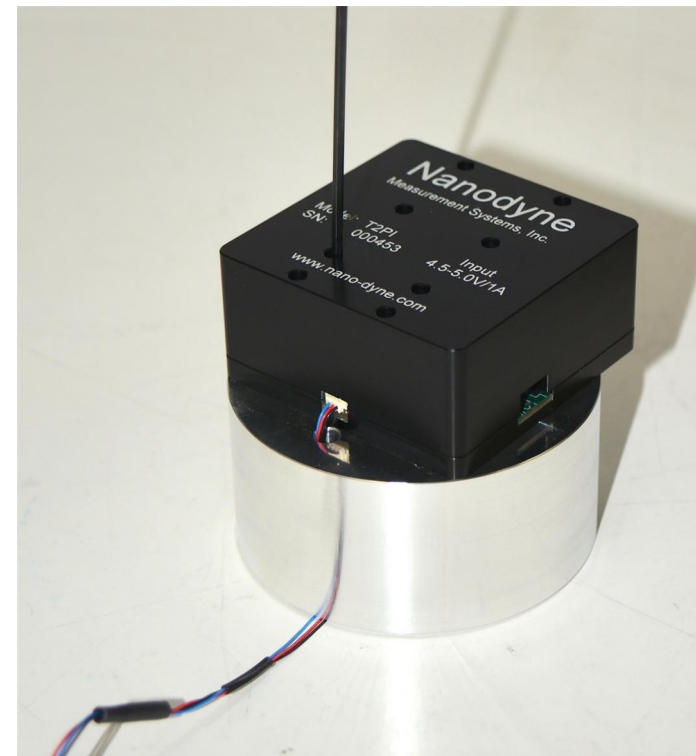
(5) Connect the illuminator to the adapter with the four 2-56 screws. Pull any excess cable back into the microscope neck.
