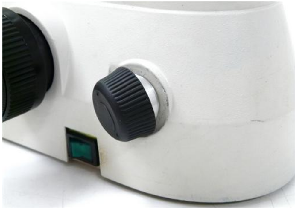
(1) Remove the rubber cover from the intensity control knob to access the setscrew. This will take some force.
