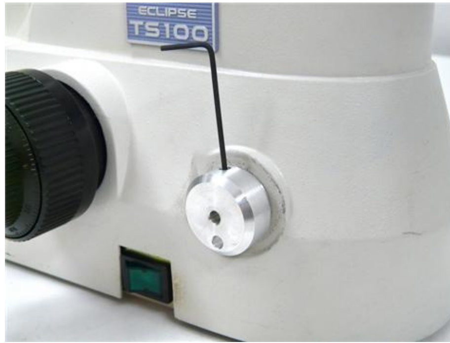
(2) Remove the metal knob by loosening the setscrew using the hex key provided.
