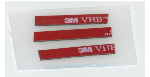
Tape to secure wires.
